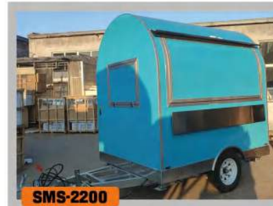
SMS-2200 Dimension(Only body) · 2200x1650x2350mm · 7.21*5.41*7.7ft Weight · 550KG/1212LB
