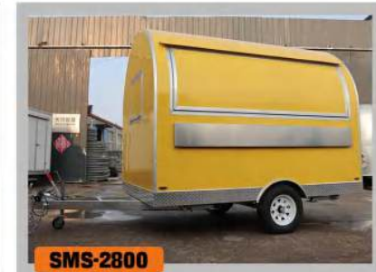
SMS-2800 Dimension(Only body) · 2800x2000x2350mm · 9.18*6.56*7.7ft Weight · 650KG/1433LB
